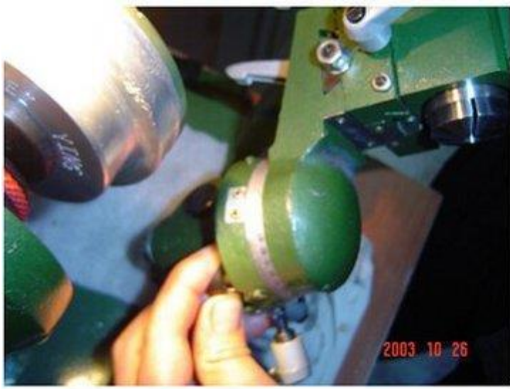
P1. uprooted limit screws can be turned around 360 degrees rotating turret, convenient grinding mill cutting edge. ♡
