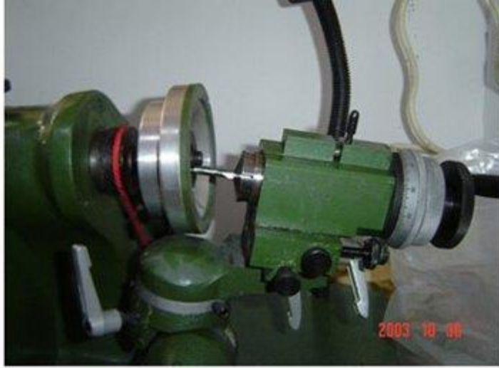
P2 .Chuck R8 with the original turret milling toolholder clamping Department of grinding knife cutting edge can be transferred to the location exhausted grinding tool turned around 45 degrees or 90 degrees the other teeth grinding
